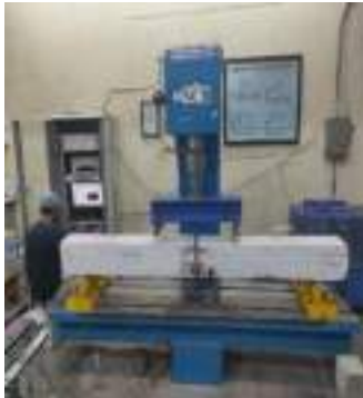
Test set up for testing of RGC beam in four-point bend test
