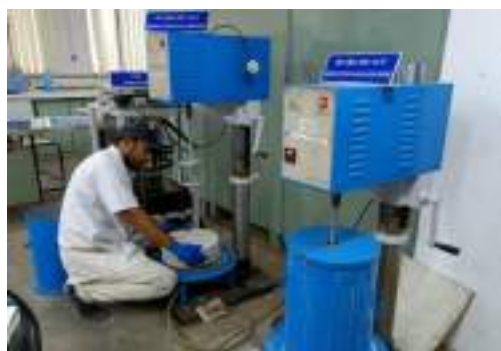
Under water Abrasion on Hardened Concrete
