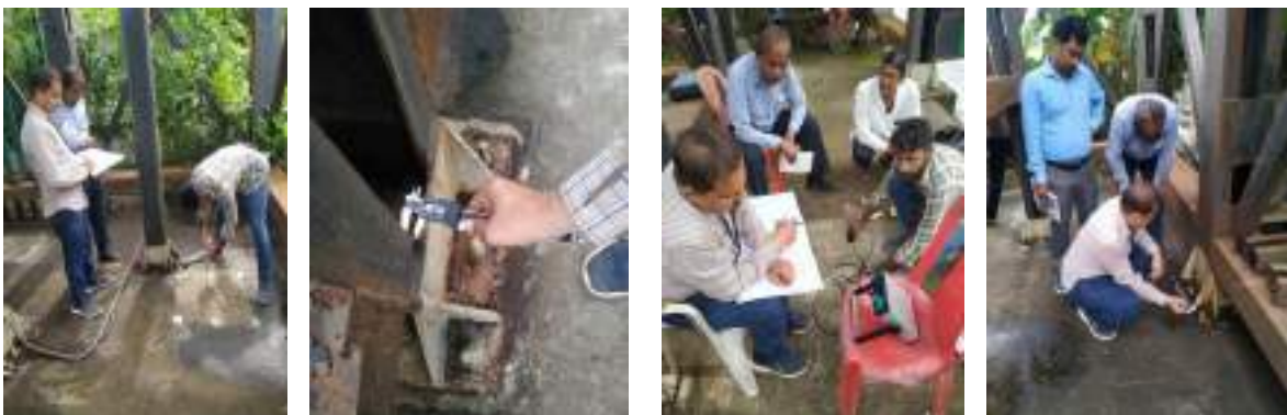
SAR (NDT) Testing of Steel Water Tank at Puri, Odisha
