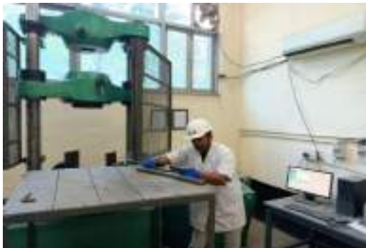
Universal testing machine- 1000kN for testing of reinforcement steel
