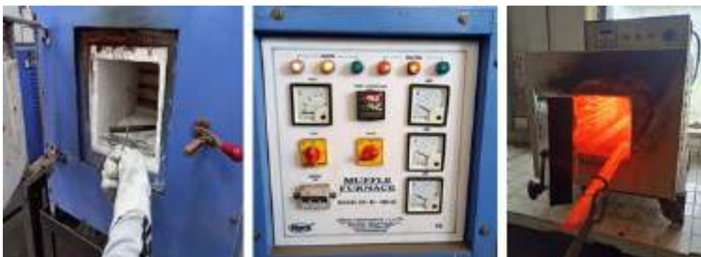
Sample of reinforcing bars kept in furnace
