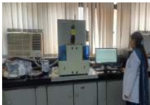
Mercury Intrusion Porosity equipment for checking porosity of concrete
