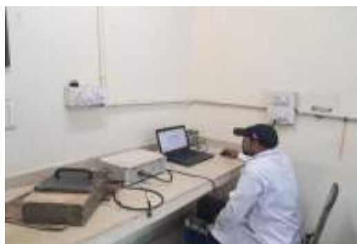
Corrosion Rate using Electrochemical Impedance Spectroscopy
