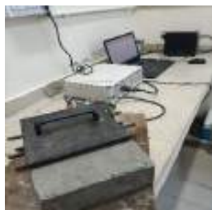
Measurement of corrosion rate using LPR
