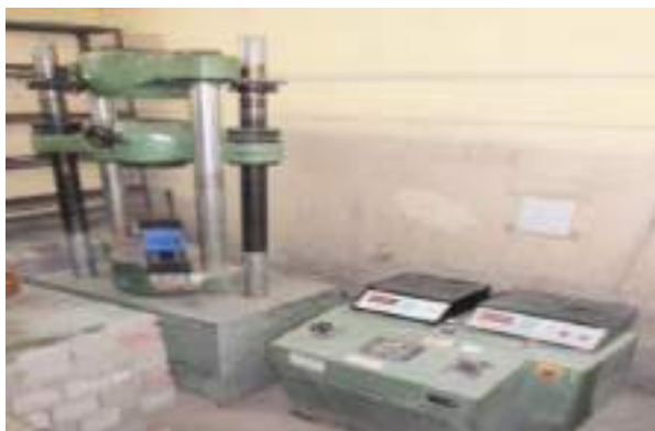
Universal Testing Machine for Reinforcement Testing facility at NCB Ahmedabad Unit
