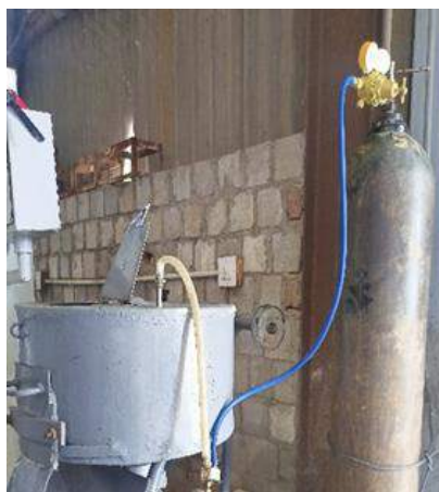
An experimental setup prepared for injecting CO 2 in fresh concrete
