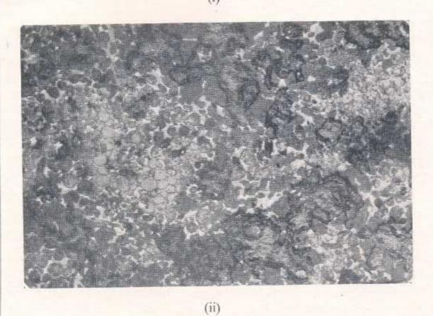
Plate 1 Photomicrograph (×280) of clinkers produced with (i) Coke Breeze (ii) SLV Coal
