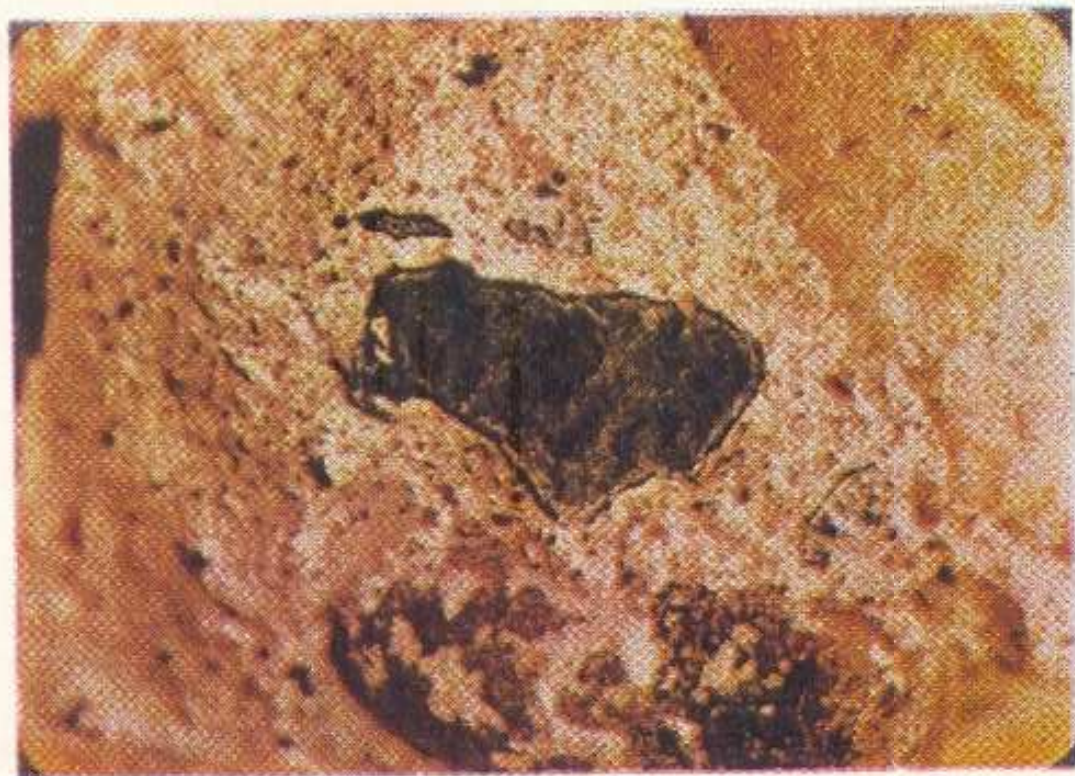
Fig 3 Dark reaction rims on aggregate
