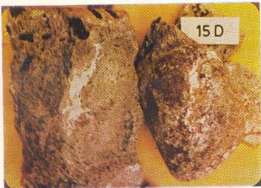
Fig 2 Gel formation on the aggregate
